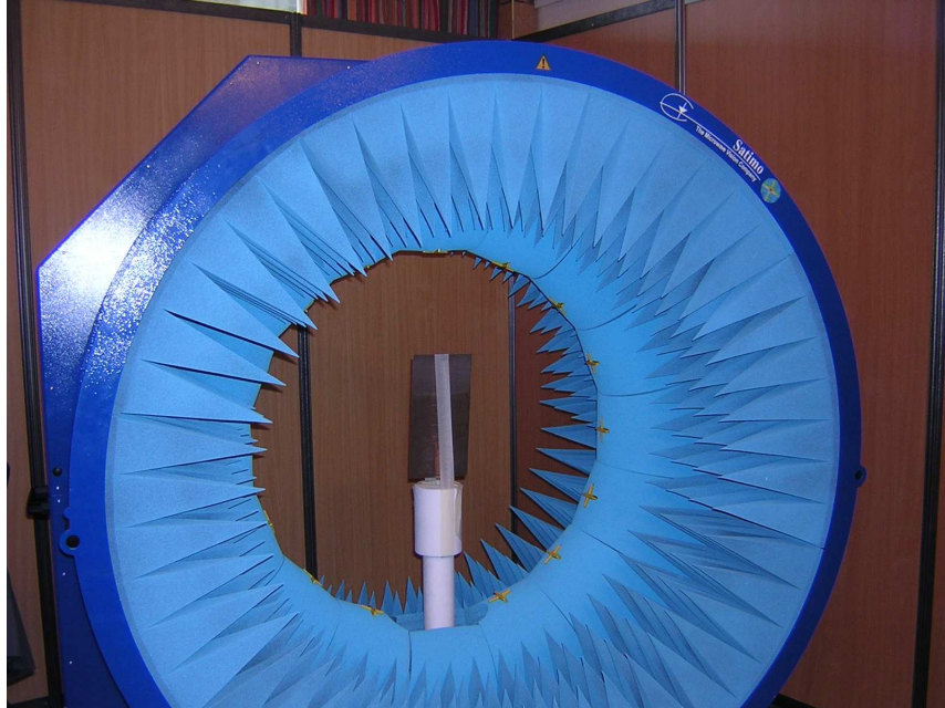
Figure 5.10: Antenna under test for radiation pattern measurement(StarLab).
