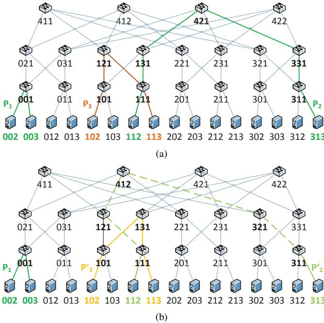
Fig. 4. FatTree topology with 16 hosts. (a) Path  $P_3$  can be inserted without migrating the paths  $P_1$  and  $P_2$ . (b) Path  $P'_3$  can only be inserted when migrating the path  $P_2$  to  $P'_2$  through DFM. The SDN controller computing and deploying appropriate rules for FM is omitted for clarity.
