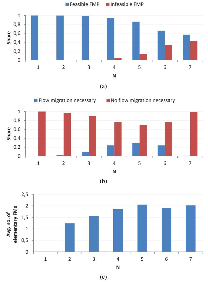
Fig. 6. (a) Share of (in-)feasible FMPs, (b) share of feasible FMPs where FM is (un)necessary, and (c) average number of elementary FMs if FM is necessary, as a function of the number  $N$  of source-destination pairs.
