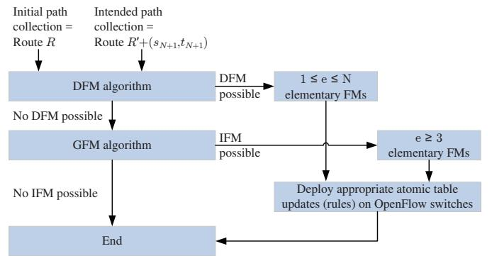
Fig. 3. Flowchart of the execution of the proposed algorithms by an SDN controller.
