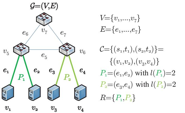
Fig. 1. Example network topology including source-destination pairs and paths.
