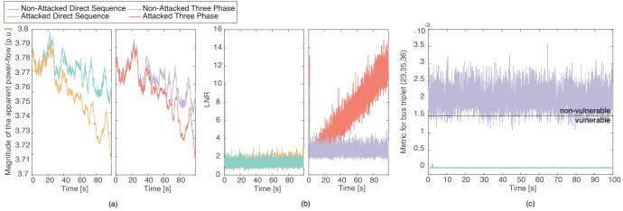
Fig. 5: Unbalanced system, attack on {23,35,36}: (a) Magnitude of the power-flow on the line between buses 21 and 22, with and without an attack on the direct-sequence and three-phase measurements; (b) LNR values with and without an attack: the attack is undetected using the direct-sequence model but is detected with three-phase estimation; (c) Vulnerability metric: the direct-sequence metric shows vulnerability and the three-phase metric is above the triplet-vulnerability threshold.
