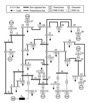
Fig. 1: PMU deployment on the IEEE 39-bus benchmark system.
