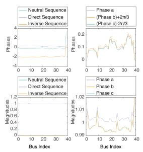
Fig. 2: Voltage phasors in a balanced system, phase representation and symmetric components, obtained after load-flow calculation at a single time instant
