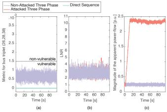
Fig. 6: Undetectable attack on the three-phase unbalanced measurements of buses {26,28,38}: (a)Vulnerability metric: both metrics are always below the triplet-vulnerability threshold; (b) Results of the LNR test with and without the attack are hardly distinguishable; (c) The attack results in a one order of magnitude misestimation of the magnitude of the power-flow on the transmission line between buses 26 and 28.
