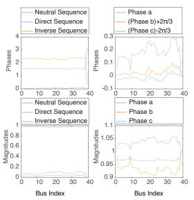
Fig. 4: Real unbalanced voltage phasors after the load flow at one time-instant according to the complete-sequence and three-phase models.
