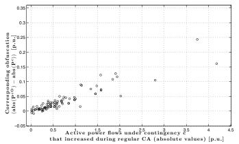
Fig. 8. Obfuscated power flows under the contingency vs. power flows that increased due to the contingency with the regular CA. Most of the obfuscated power flows exceed the actual power flows.
