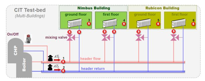
**Adversary:** Infect some field devices with malware ( $\dot{a}$  la Stuxnet) corrupting measurements sent to PLCs (Here:  $AT_1$  and  $AT_2$ )
