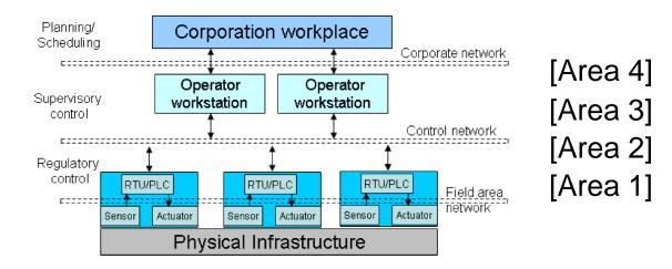
Figure 1. Architecture of control systems.
