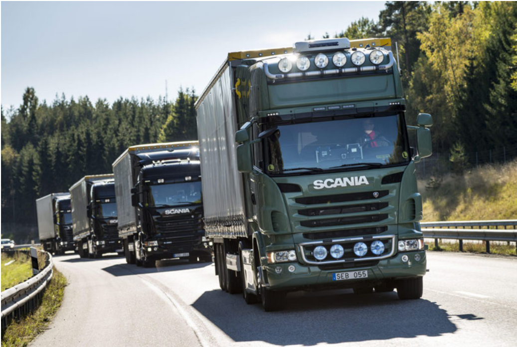
Figure 1.7: An HDV platoon traveling with a given initial set speed and relative distance. Several external forces such as air drag, road friction and gravity along with internal forces affect a vehicle in motion. (Photo provided courtesy of Scania CV AB.)
