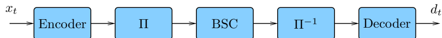
Figure 5.2: Block-diagram for the communication over a BSC. The symbol \Pi is a notation for the IA unit.
