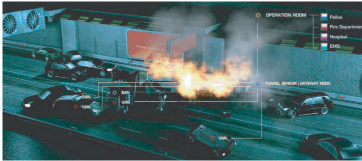
Figure 1.5: A tanker has caught fire in a road tunnel and an embedded sensor network supports the rescue personnel with dynamic information about the accident site. (Copyright: RUNES)
