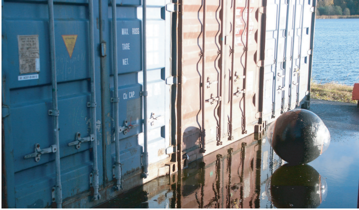
Figure 1.1: A spherical UGV patrolling a container storage. The transparent windows on each side house cameras, providing a 360° view around the robot. (Copyright: Rotundus AB)
