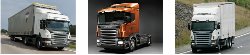
Figure 5.2: Test vehicles used for road tests of the grade estimation algorithm. Three vehicle configurations were used. Starting from the left they were a tractor-semitrailer combination (A), tractor only (B), and rigid truck (C). (Photographs courtesy of Scania CV AB)
