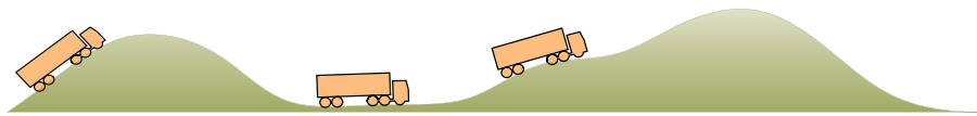
Figure 2.5: HDVs traveling on a hilly road. At the position of the leftmost vehicle, it is advantageous to lower the speed to take full advantage of the upcoming downhill road segment. In the second position the overall fuel economy can be improved by increasing the speed before the steep part of the hill is reached. In the third position it is important to maintain the driving torque, to avoid costly loss of turbo pressure when entering the continued ascent.
