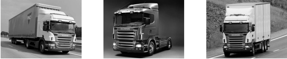
Figure 5.2: Test vehicles used for road tests of the grade estimation algorithms. Three vehicle configurations were used. Starting from the left they were a tractor-semitrailer combination (A), tractor only (B), and rigid truck (C). (Photographs courtesy of Scania CV AB)
