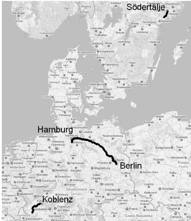
Figure 6.2: Map showing the locations of the road segments used in the estimation convergence study. The reference road profiles for the segments Södertälje–Norrköping and Koblenz–Trier are based on experimental data collected on the ground. The Hamburg–Berlin segment reference grade was determined from NASA SRTM data. (Image courtesy of Google)
