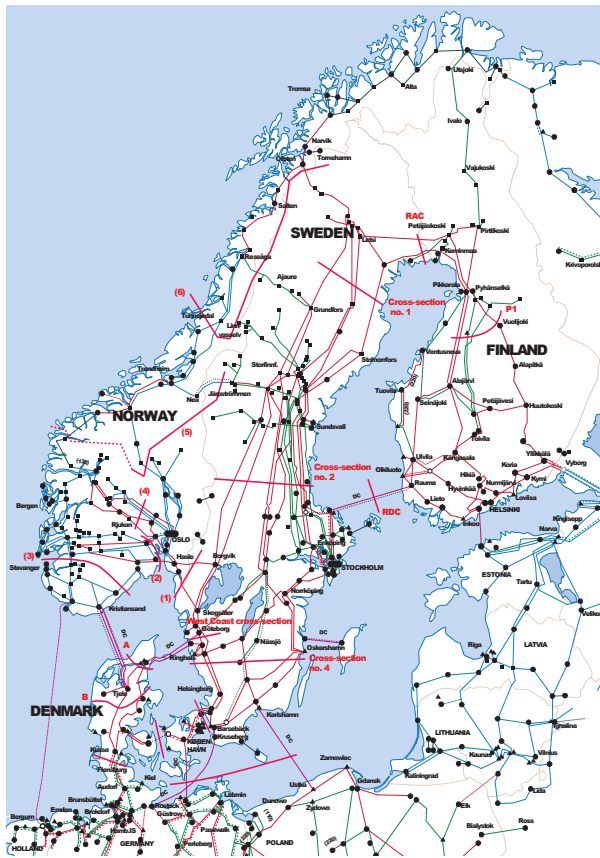
(b) The Nordic power transmission grid
