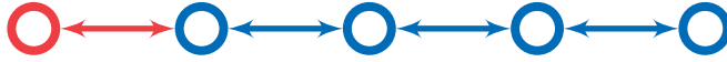
Figure 3.1: System configuration with a line graph topology. The red node denotes the faulty agent, while the blue nodes denote the followers.
