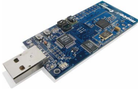
Figure 1.4: A Tmote Sky low power wireless sensor module, used for wireless sensor network applications (Courtesy of Moteiv).
