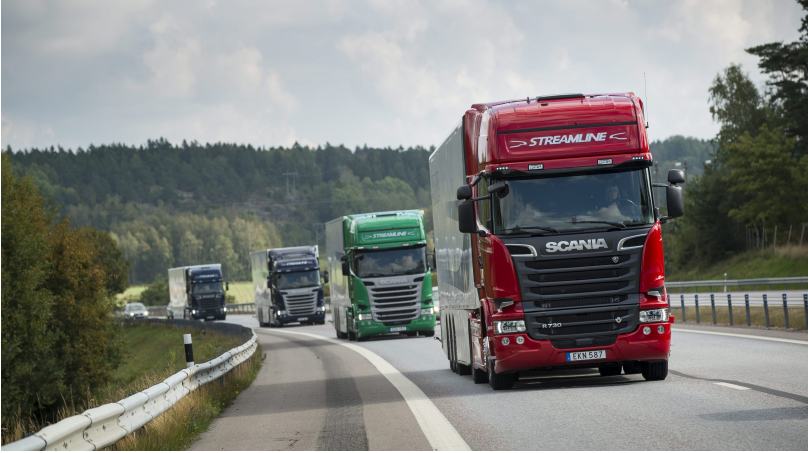
Figure 1.3: Four-vehicle platoon driving over an uphill stretch. Photo provided by courtesy of Scania AB.
