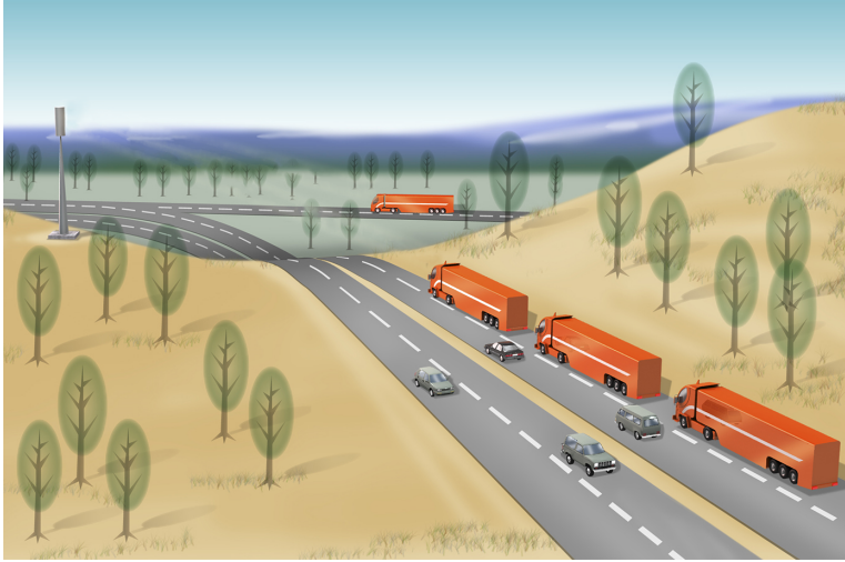
Figure 1.6: Illustration of a heavy-duty vehicle platoon driving on a public highway. Because of vehicle heterogeneity, altitude variations can significantly affect the platoon fuel consumption. Furthermore, external traffic can interfere with platoon operations.
