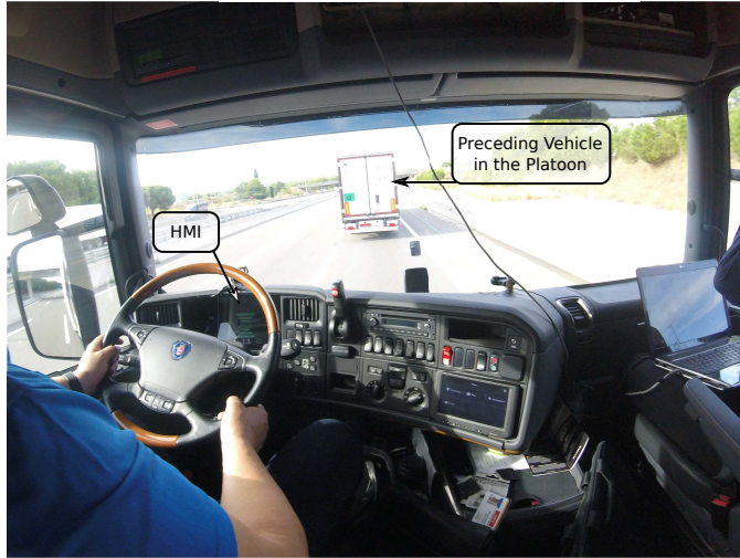
Figure 8.15: View from the cockpit of the green vehicle while trailing the blue vehicle in the platoon. The on-board HMI can be seen in the dashboard. The computer on right side of the image is used to monitor and collect data from the on-board system.
