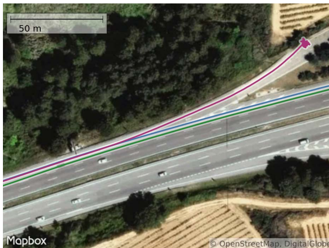
(b) At the second merge point, the starting position of the red vehicle is located on the upper right of the image on a parking lot next to the highway. The lack of an acceleration lane made it necessary to start before the scheduled departure time.
