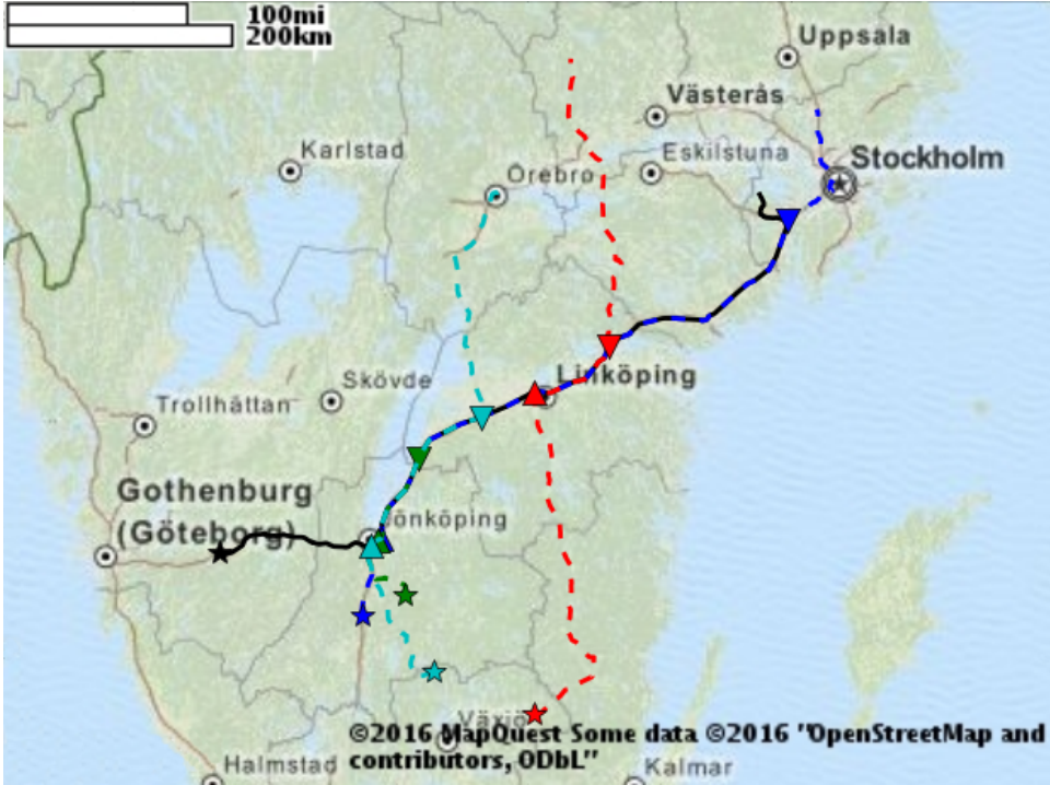
Figure 6.8: The routes of a platoon coordinator with four coordination followers. The route of the coordination leader is shown in black, the routes of the coordination followers are dashed. The beginning of a route is marked with a star. The merge point of a follower is indicated with an upwards-facing triangle and the split point with a downwards-facing triangle.
