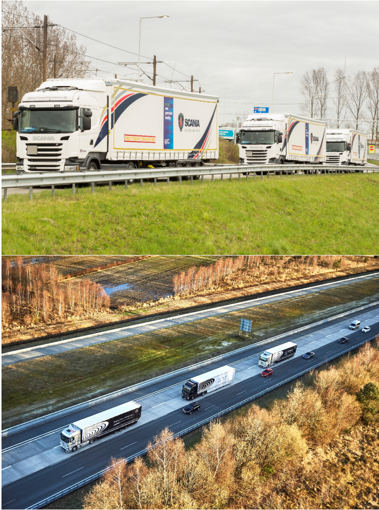
Figure 1.1: Platooning demonstrations in the scope of the European truck platooning challenge 2016. (Image source: European Truck Platooning Challenge)
