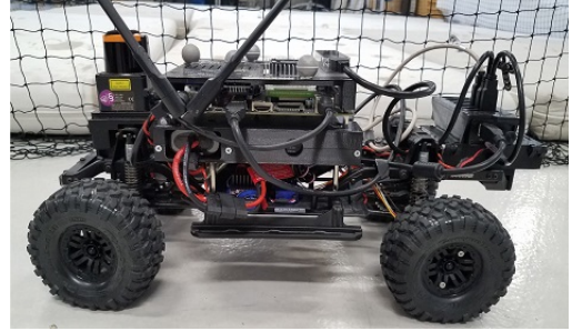
Fig. 5: SVEA vehicle based on an NVIDIA Jetson TX2 embedded computer used to evaluate the proposed solutions.
