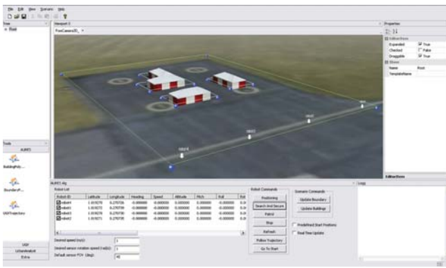
Fig. 11. The AURES operator console. The operator can choose which task should be launched. It is also possible to change scenario parameters such as the speed of the robots and coordinates of the map. The map shows the location of the robots.
