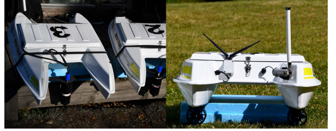
Fig. 3. ASVs used in the experiments. The left and right pictures show the front and back of the “ducklings,” where the acoustic receivers and thrusters, RFD868 and Wifi antennas can be seen, respectively.
