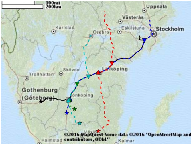
Fig. 6. The routes of a platoon coordinator with four coordination followers. The route of the coordination leader is shown in black, the routes of the coordination followers are dashed. The beginning of a route is marked with a star. The merge point of a follower is indicated with an upwards-facing triangle and the split point with a downwards-facing triangle.
