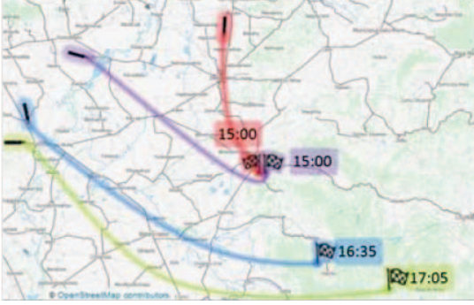
(a) Four different HDVs from different companies need to be coordinated for platooning.
