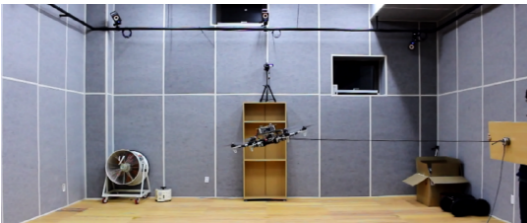
Fig. 11. Experimental set-up of a DOB-applied UAV with an elastic tether to apply an outer lateral disturbance and a load cell to measure the disturbance force.
