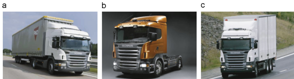
Fig. 2. The proposed road grade estimation algorithm has been tested on highway E4 between Södertälje and Nyköping, Sweden, using three types of HDVs. Starting from the left they were a tractor-semitrailer combination (A), tractor only (B), and rigid truck (C). (Photographs courtesy of Scania CV AB.)
