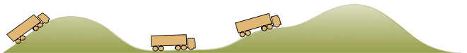
Fig. 1. HDVs traveling on a hilly road. At the position of the leftmost vehicle, it is advantageous to lower the speed to take full advantage of the upcoming downhill road segment. In the second position the overall fuel economy can be improved by increasing the speed before the steep part of the hill is reached. In the third position it is important to maintain the driving torque, to avoid costly loss of turbo pressure when entering the continued ascent.
