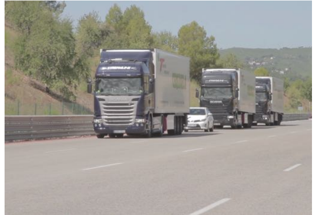
Fig. 1. A human-driven car has cut in between two trucks in the platoon. Such interference may happen if the human is subject to danger in its own lane (e.g., blocked lane by road work), but should in non-critical situations be discouraged due to performance degradation of the platoon.
