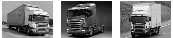
Fig. 1. The vehicle types used for verification. Starting from the left a tractor-semitrailer combination (A), tractor only (B), and rigid truck (C) were used.
