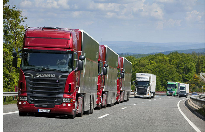
Fig. 1. Heavy duty vehicles traveling in a platoon can achieve significant fuel reduction. Preview information in hills should be taken into consideration for improved fuel-efficiency.
