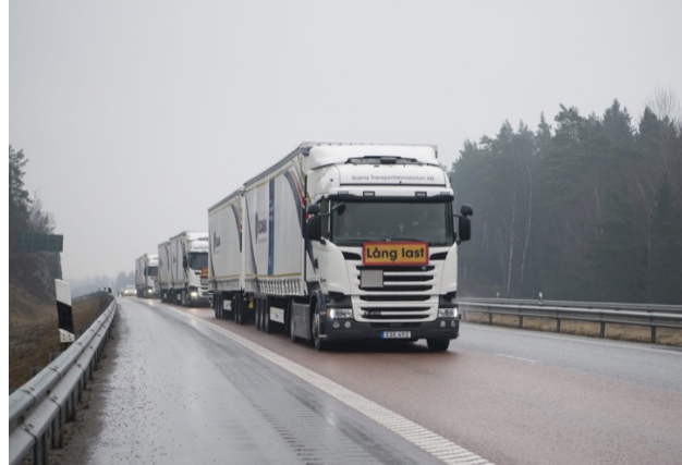
Fig. 1: Three Scania trucks platooning from Södertälje, Sweden, to Rotterdam, the Netherlands, during the European truck platooning challenge.
