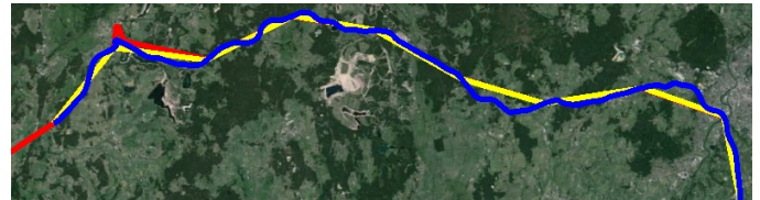
Fig. 6. An example of a vehicle's raw probe data (red line), map-matched data (yellow line), and the inferred path (blue line). Notice that some probe data are outside the road network and could therefore not be map matched, however the path inference managed to find a path between all map-matched points.
