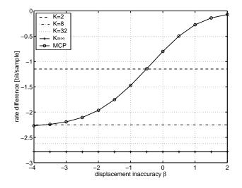
**Fig. 6.** Rate difference to intra-frame coding vs. displacement inaccuracy for a group of K pictures. The displacement errors are maximally correlated ( $\rho_{\Delta} = 1$ ) and the residual noise is -30 dB. For reference, the performance of motion-compensated prediction with optimum Wiener filter is also plotted.
