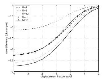
Fig. 5. Rate difference to intra-frame coding vs. displacement inaccuracy for a group of K pictures. The displacement errors are correlated with  $\rho_{\Delta} = 0.5$  and the residual noise is -30 dB. For reference, the performance of motion-compensated prediction with optimum Wiener filter is also plotted.
