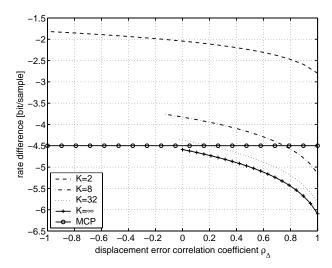
**Fig. 4.** Rate difference to intra-frame coding vs. displacement error correlation coefficient for a group of K pictures. Very accurate motion compensation is assumed ( $\beta = -4$ ) and the residual noise is -50 dB. For reference, the performance of motion-compensated prediction with optimum Wiener filter is also plotted.
