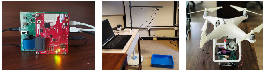
(a) IWR1843boost mmWave sensor with DCA1000evm data capture card. (b) Water detection setup in a Lab environment. (c) mmWave sensor mounted on a DJI Phantom 4 Standard drone.
